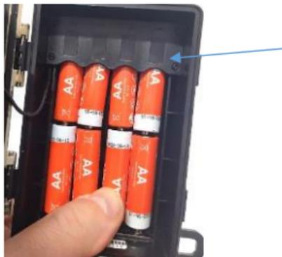
**Note 1:** Do Not mix old and new batteries together in the camera
