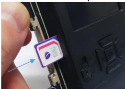
The camera supports SIM card with LTE 4G High Speed. If original pictures or videos are sent, minimum Upload Speed 5MB/sec is required
