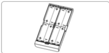
Insert 8pcs of new alkaline batteries according to the +/- directions shown on the bottom of the battery compartment
