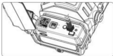
Press the "Eject" button to eject the battery compartment
